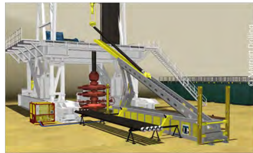
Catwalk machine to lift pipe for the ground racks
